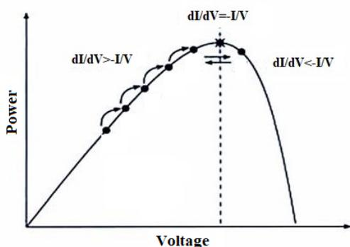
**Fig. 4.** The principle of the IC algorithm.
