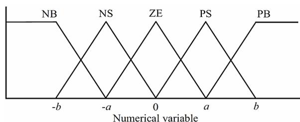
**Fig.5.** The proposed membership function for inputs and output of the fuzzy logic algorithm.
