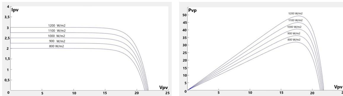
Fig. 6. I-V and P-V characteristics of the modeled PV panel under variable irradiance levels.
