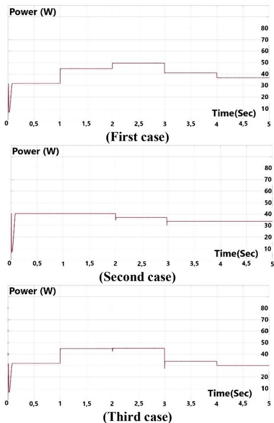
Fig. 13. Output power of solar panel with IC algorithm.
