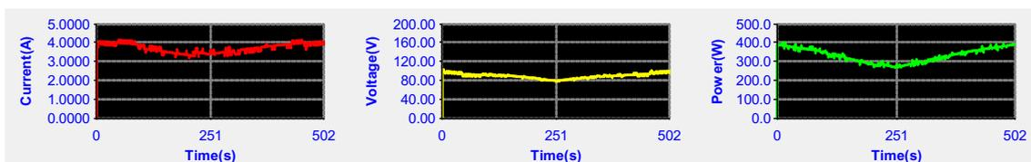
Fig. 19. The current, voltage and power values obtained by using P&O algorithm in the third stage
