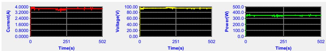
Fig. 17. The current, voltage and power values obtained by using P&O algorithm in the first stage
