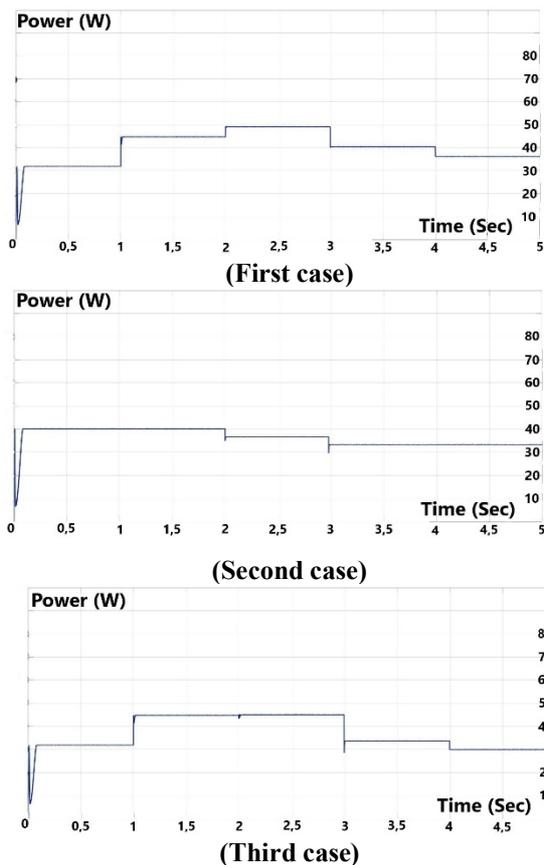
Fig. 12. Output power of solar panel with P&O algorithm.
