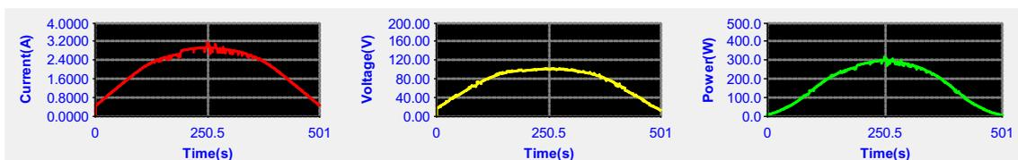
Fig. 21. The current, voltage and power values obtained by using IC algorithm in the second stage
