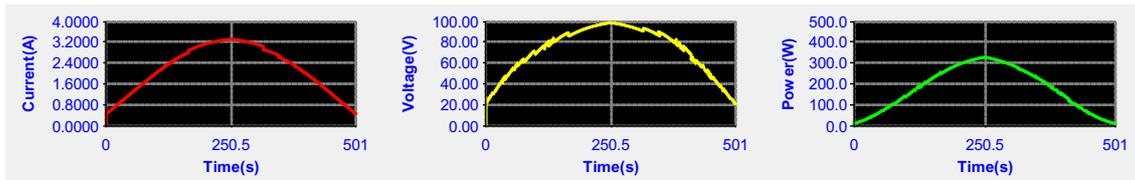
Fig. 24. The current, voltage and power values obtained by using FL algorithm in the second stage
