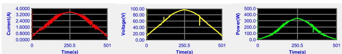
Fig. 18. The current, voltage and power values obtained by using P&O algorithm in the second stage
