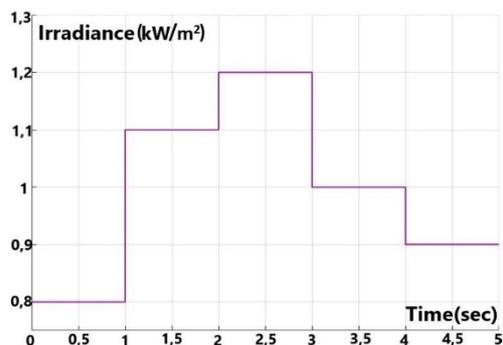
Fig. 9. The different levels of solar irradiance.
