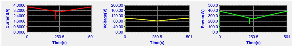
Fig. 25. The current, voltage and power values obtained by using FL algorithm in the third stage
