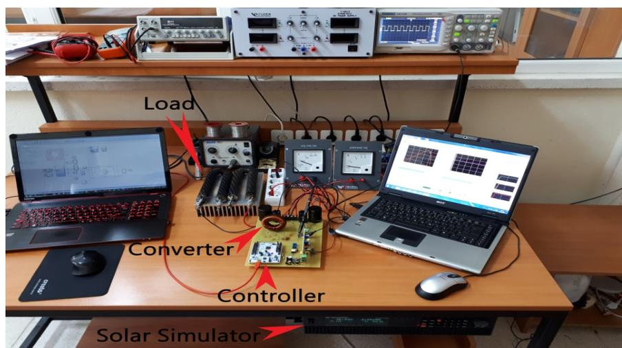
**Fig. 15.** The hardware arrangement of the system.
