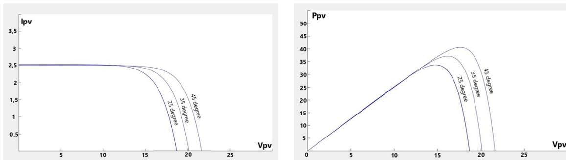
Fig. 7. I-V and P-V characteristics of the modeled PV panel under variable temperature levels.
