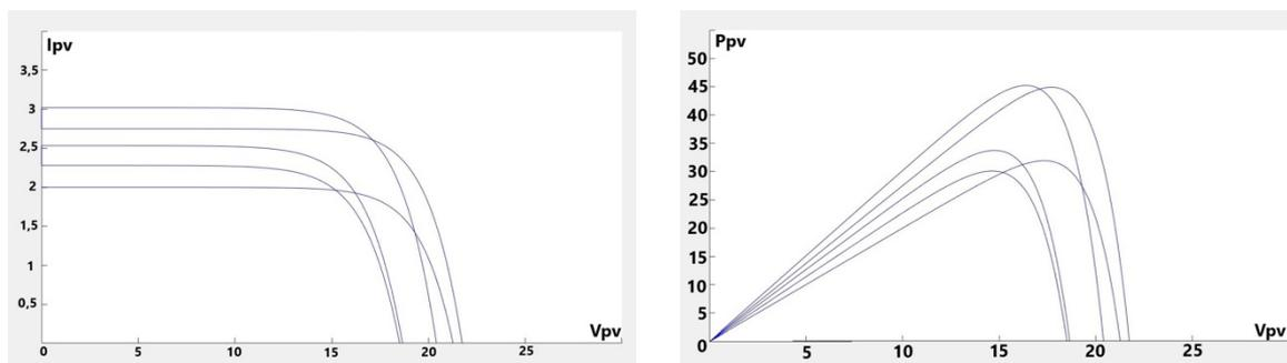
Fig. 8. I-V and P-V characteristic of the modeled PV panel under variable temperature and variable irradiance levels.
