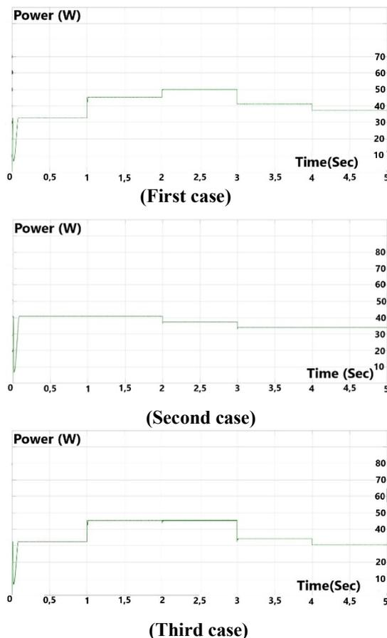
Fig. 14. Output power of solar panel with FL algorithm.
