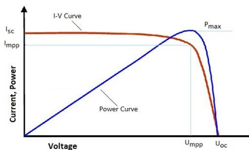
Fig. 1. P-V & I-V characteristics of a solar panel.
