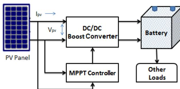
Fig. 3. Typical diagram of MPPT in a PV System
