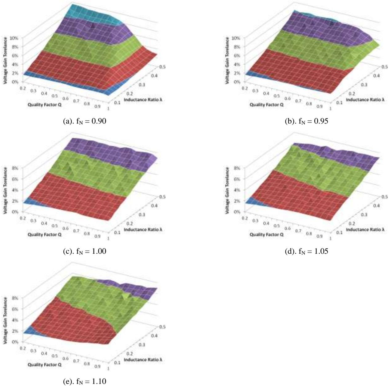
**Fig. 4.** Tolerance of voltage gain vs quality factor and inductance ratio taking normalized frequency as a parameter about three-level LLC converter.
