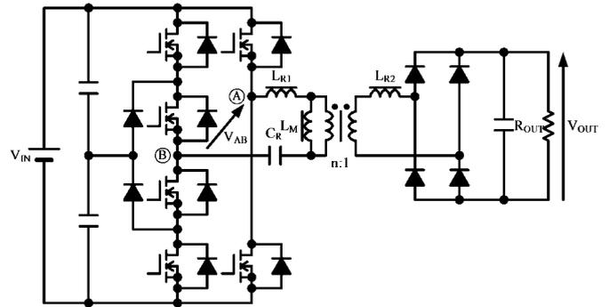
**Fig. 1.** Hybrid full-bridge three-level LLC resonant converter.
