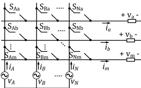
Fig. 2. Conventional  $m \times n$  matrix converter.
