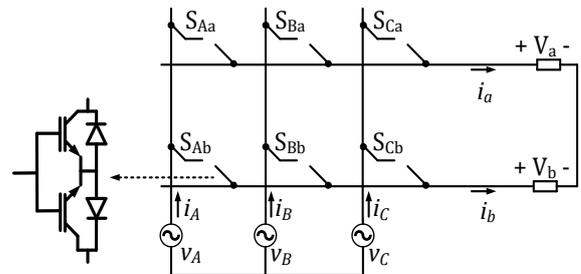
Fig. 3. Three-phase to two-phase matrix converter.
