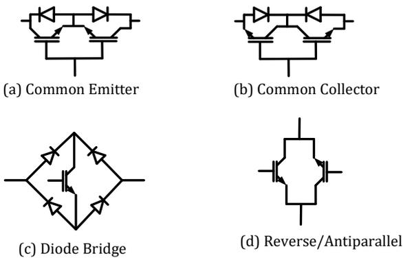
Fig. 8. Bidirectional switch configuration.
