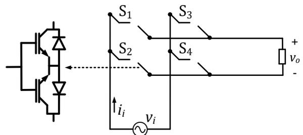
Fig. 5. Single-phase to single-phase matrix converter.
