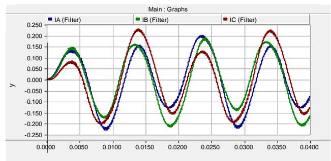
Fig. 22. Source current waveform (after low-pass filter).
