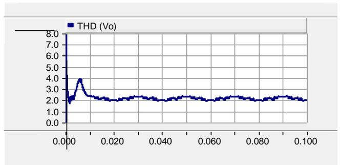
**Fig. 15.** Total harmonic distortion of load voltage.
