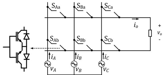
Fig. 4. Three-phase to single-phase matrix converter.
