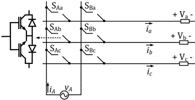
Fig. 6. Single-phase to three-phase matrix converter.
