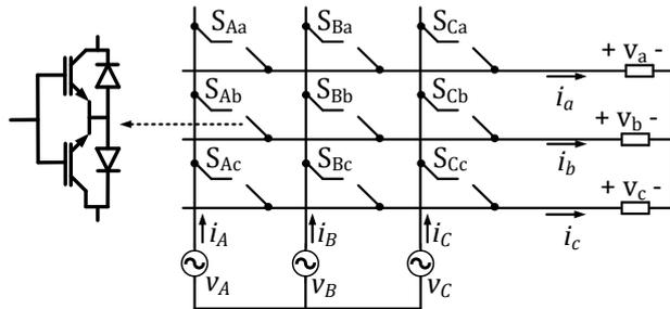
Fig. 7. Three-phase to three-phase matrix converter.
