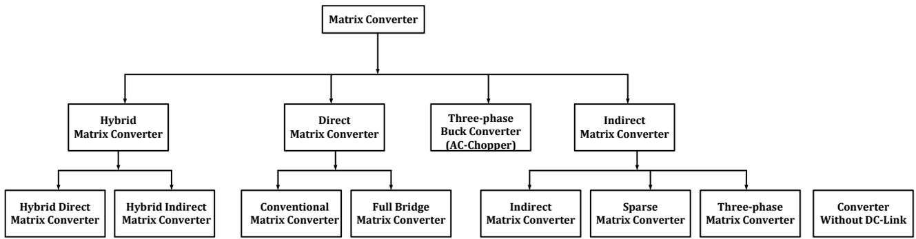
Fig. 1. Classification of matrix converter.
