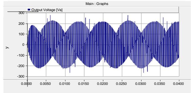
Fig. 19. Phase A load voltage waveform.
