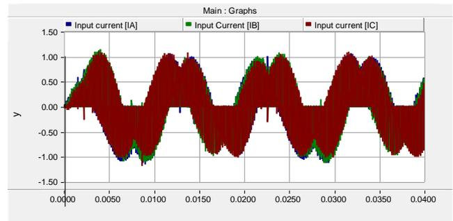
Fig. 21. Source current waveform (before low-pass filter).
